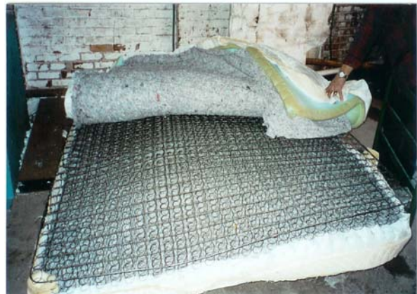
Conigliaro Industries, Inc. puts low-quality mattresses through a shredder (above), which separates the polyurethane foam from other materials. Below, brand name mattresses usually are filleted on each side and then run through the shredder, allowing the company to recycle a higher portion of material.
